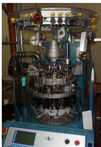
Figure 1. Automatic stocking knitter Lonati 462 3 3/4" used for production of men, women and children's stockings.
