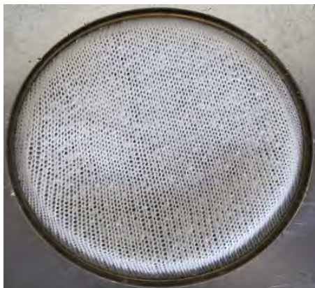
Figure 3. Photo of cotton sock after 10000 rotations in the in the direction of rows.
