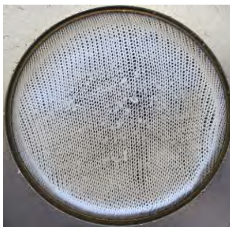
Figure 5. Photo of cotton sock after 4000 rotations in the in the direction of rows
