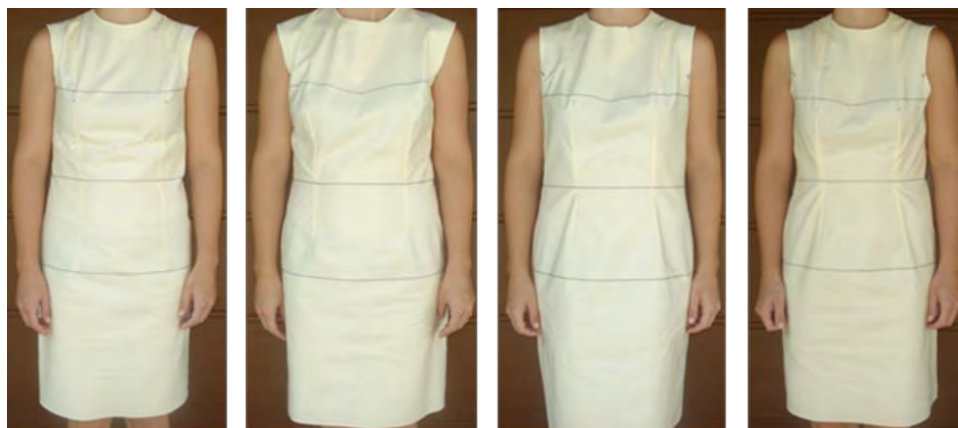
Figure 5: Front side of the basic pattern: a. System 1, b. System 2, c. System 3, d. System 4
