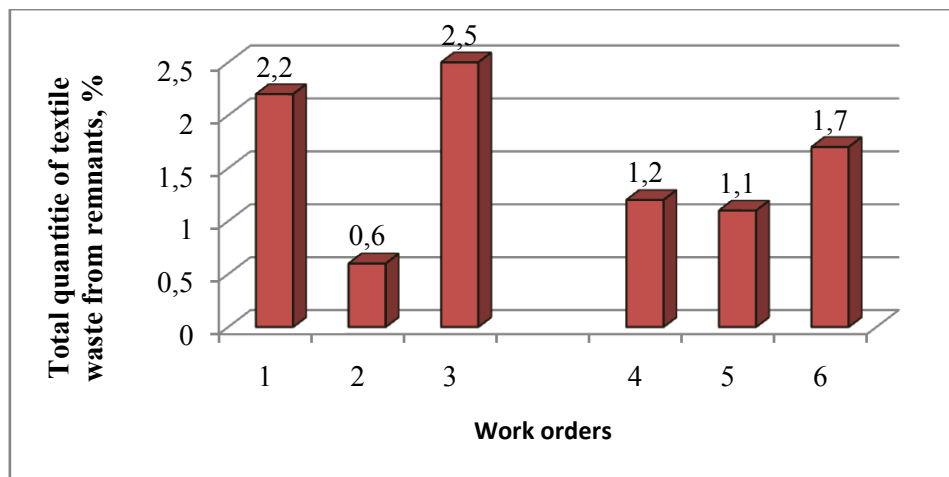
Figure 2. Total quantities of textile waste from remnants in production companies A and B, %
