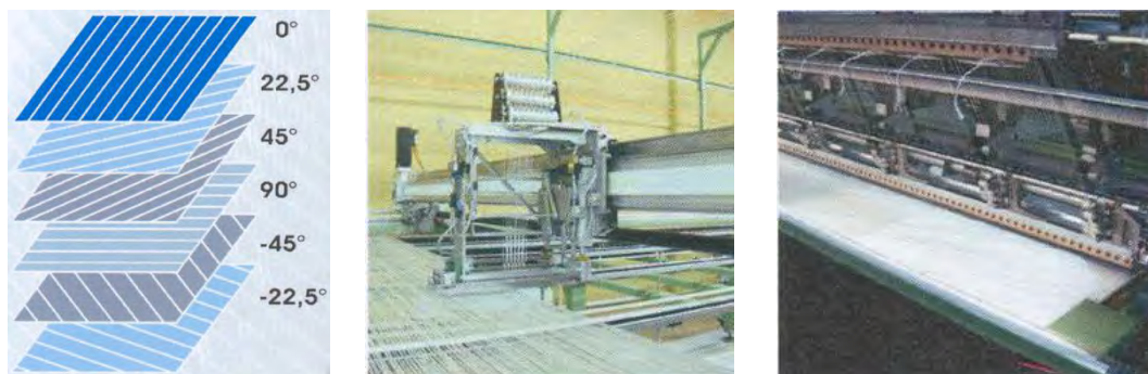
Fig. 4. Possible angles geotextile weaving looms and appearance [7]
