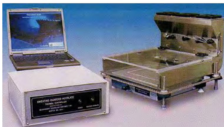
Figure 2. Device for measuring resistance of water vapour flow (Ret)
