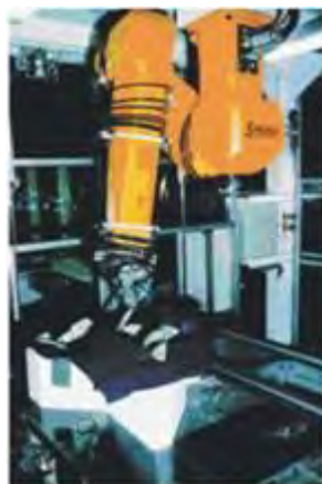
Figure 1. Industrial robot with a water jet cutting textile materials
